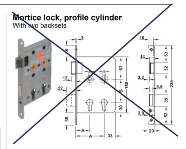
The lock is particularly suitable for doors that are supposed to close as tightly as possible. Direct connection with the door leaf is avoided. The two consecutive backsets allow the use of half fitting sets and single cylinders. Only drillings that do not penetrate the door panel and are not positioned on one axis are required on each side of the door.
